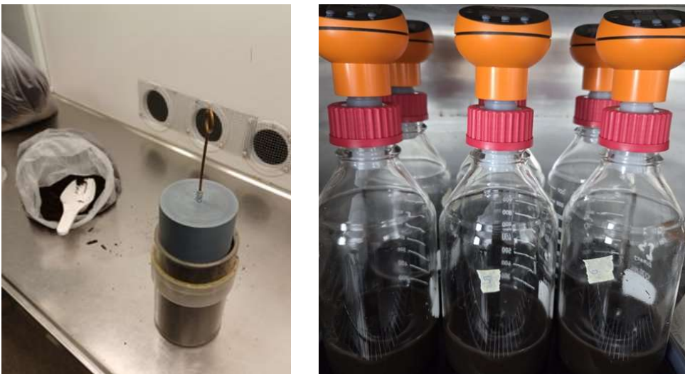
Figure 3. Examples of testing measurands including bulk density measurement (left) and stability (OUR) measurement (right).
